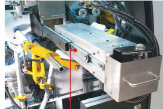
Pullout design for easy bulb change and maintenance.
